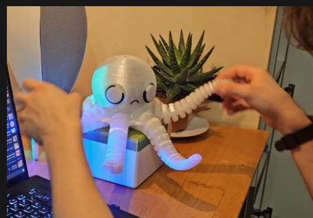
soft-robotic TPU tentacles can be interacted with to act out different emotions
